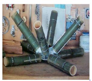
Connection with steel wire
