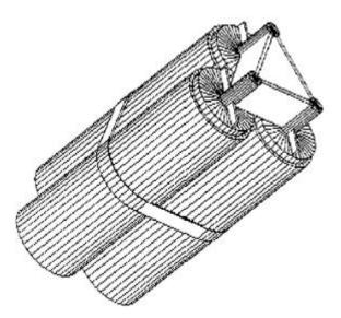
Cane bundles must be used for bigger loads. When using them for construction a possible connection can be achieved by projeting steel tips out of a wood cylinder (see interlocking connection), so that these tips can be welded to a plate or any other cetral component, to fix the relative position of the canes.
