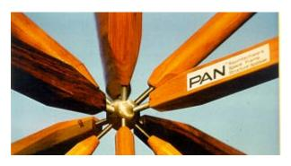
Pan-spacetruss. Small bamboo canes (diameter up to 80mm) can transfer ca.50% of the maximal tensile force if threaded bars are glued or sheded into the caneends. For compressive forces the maximum force is where the cane breaks if connected with a headplate. If overhead working is necessary tests by an officially recognized material-testing-institution and special permission of the building departement are required. (germany)
